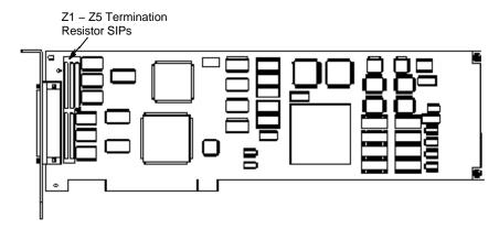
The KZPBA-CB internal termination is disabled by removing the termination resistors RM1-RM8 as shown in Figure 4–1.
